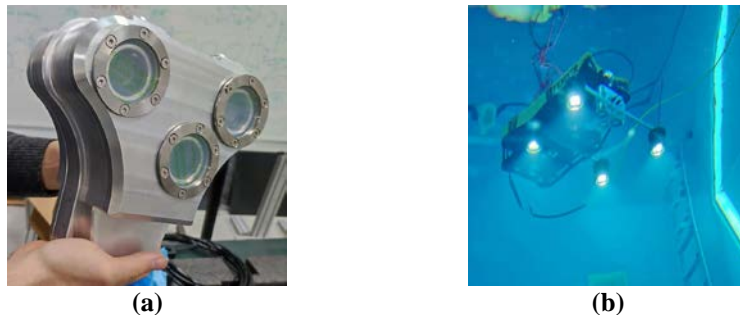
Fig. 4. Functional prototype of the optical payload (a), installed on the bottom of a professional-grade ROV (b).
